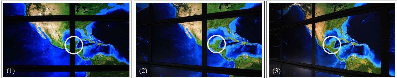
Figure 1: The grid formed by monitor bezels on wall displays is often compared to a french window. We designed two interaction techniques that transform that grid into an actual french window. On the map, (1) the Yucatán peninsula (white circle) is partially hidden by bezels. (2) With one of the techniques, GridScape, users can reveal that part of the map simply by slanting their body or moving slightly to the right. (3) Moving further right, the entire eastern coast of Mexico can be shown without any bezel occlusion.
