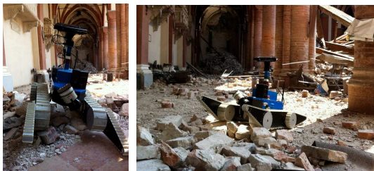
Figure 7: Urban Search and Rescue robot TALOS.
