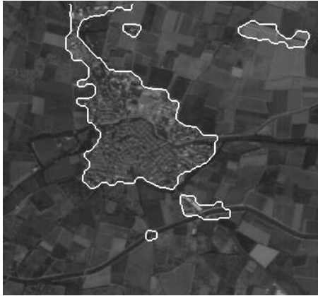
Fig. 6. Result of urban area extraction on a SPOT5 simulation of Toreilles (5 meter resolution)
