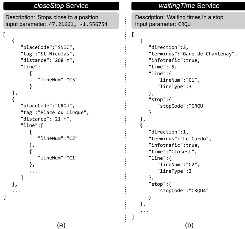
Fig. 1. JSON documents from two TAN API services: (a) the closeStop service, which returns the closest bus/tram stops to a geolocation, and (b) the waitingTime service, which returns waiting times for a particular bus/tram stop.
