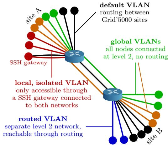
Figure 2: Types of VLAN provided by KaVLAN.
