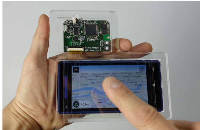
Figure 1: Our transparent electric field sensing design can be placed on top of a mobile device to enable 3D input and motion gestures.
