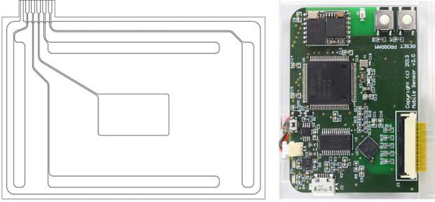
Figure 2: (a) Electrode array design, (b) drive electronics
