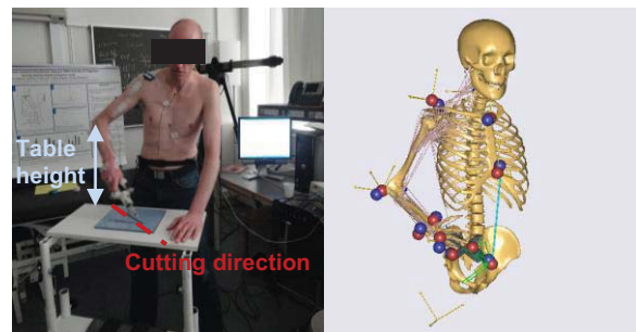
Fig 1: Real task experimental protocol and simulated task in the AnyBody software.
