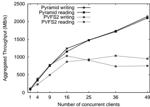
**Figure 3: Weak scalability: fixed subdomain size, increasing number of client processes**
