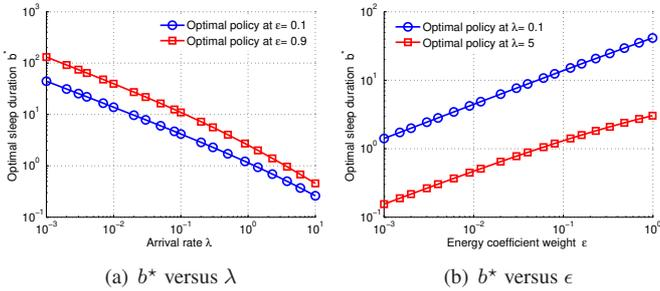
Figure 1: Optimal sleep duration with exponential off times.
