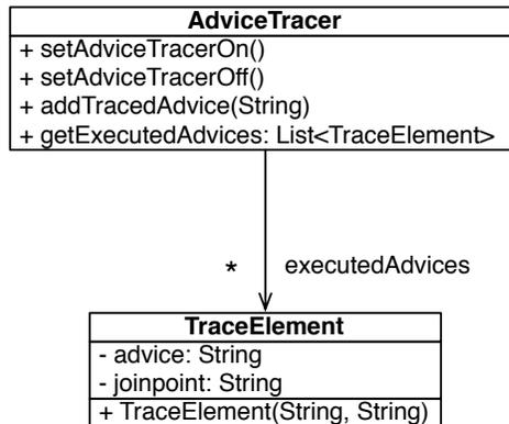
Figure 4. The class diagram of AdviceTracer.
