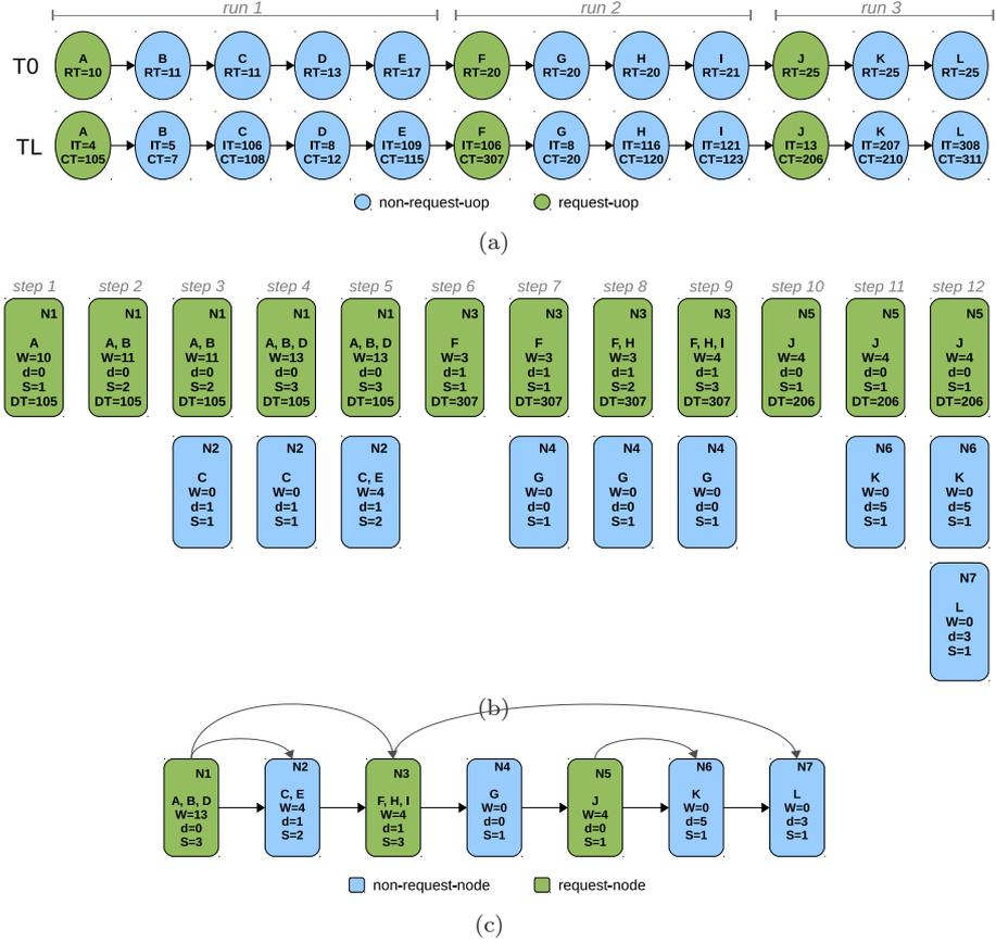
Figure 3: Example of BADCO model building : (a) Traces T0 and TL containing the same 12 dynamic  $\mu$ ops in sequential order, (b)  $\mu$ op-by- $\mu$ op processing of the traces, (c) final BADCO model featuring 7 nodes ( $RT$ =retirement time,  $IT$ =issue time,  $CT$ =completion time,  $DT$ =dependence time,  $S$ =node size,  $W$ =node weight,  $d$ =origin of the dependence edge).
