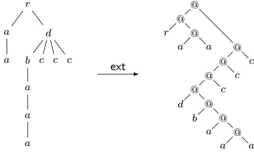
Figure 1: Curry encoding of an unranked tree.
