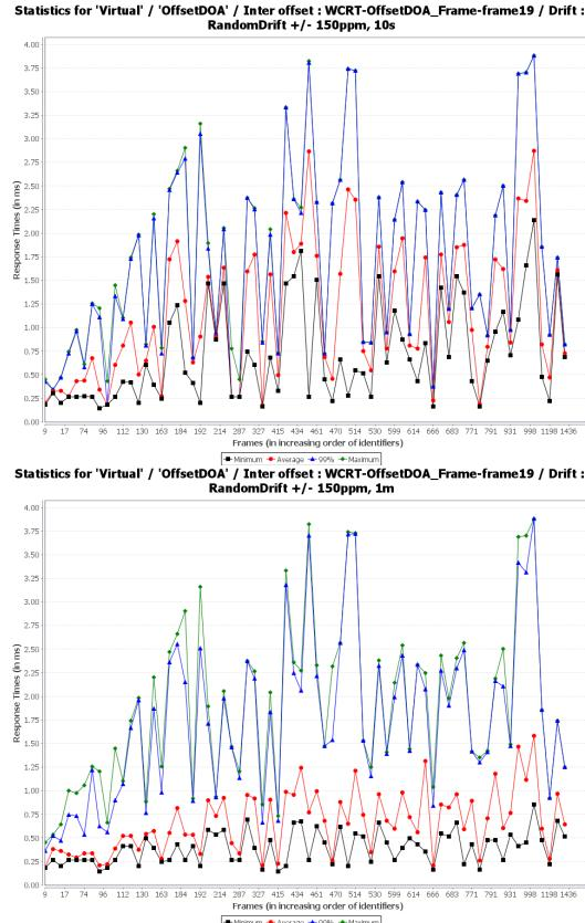
Figure 3. Simulation statistics with initial phasings leading to the worst case response time for the frame with identifier 192. The top and bottom graphics respectively show response time statistics after 10 seconds and 1 minute of simulation. Lowest to highest curves are : minimum, average, 99.9% quantile and maximum.
