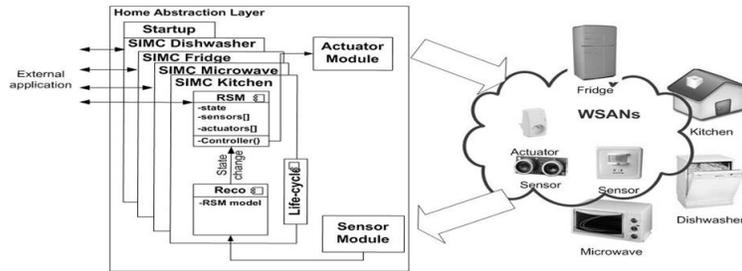
Fig. 2. SIMC architecture based upon the OSGi framework
