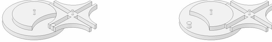
Figure 7: The Maltese Cross at two different stages of its rotation, showing how conventional interfaces change.
