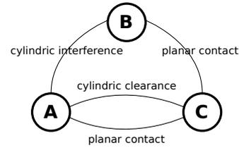
Figure 9: The CIG generated of the simple cap-screw model.
