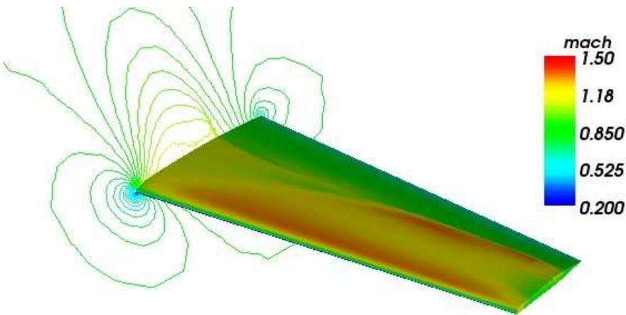
**Fig. 15** Geometrical configuration and Mach number field : a) initial aerodynamic optimum solution, and b) aero-structural Nash game solution using the orthogonal decomposition.
