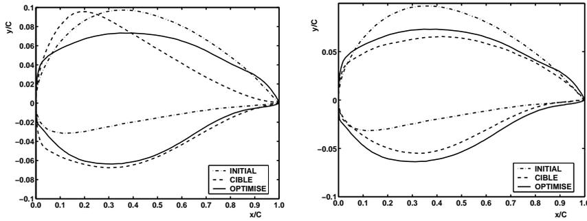
**Fig. 5** Comparison between the optimized airfoil (solid line) with the initial airfoil and the target airfoil associated with the subsonic conditions of the first point (left), and the target airfoil associated with the transonic conditions of the second point (right); from [28]
