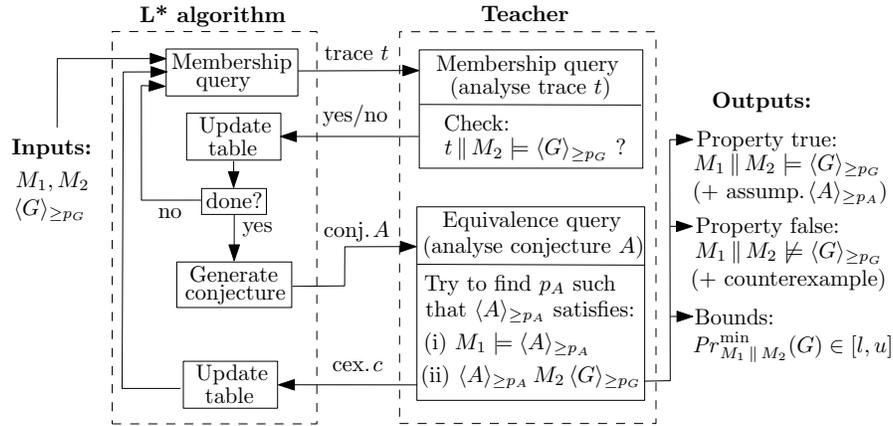
**Fig. 3.** Overview of probabilistic assumption generation [20], using an adaption of L\*: generates assumption  $\langle A \rangle_{\geq p_A}$  for verification of  $M_1 \parallel M_2 \models \langle G \rangle_{\geq p_G}$  using rule (ASYM).
