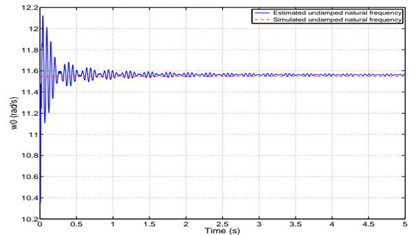
Fig. 15. Kalman filter estimates for  $\omega_0$  with SNR = 80dB and high frequency sinusoidal noise
