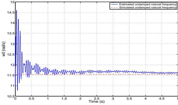
Fig. 11. Kalman-Bucy algorithm estimates for  $\omega_0$  with SNR = 50dB
