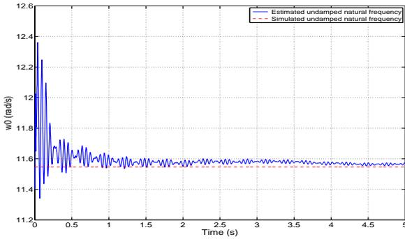
Fig. 12. Kalman-Bucy algorithm estimates for  $\omega_0$  with SNR = 80dB
