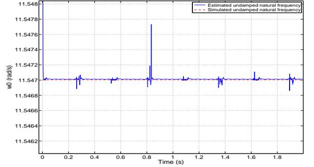
Fig. 14. Algebraic method estimates for  $\omega_0$  with SNR = 80dB and high frequency sinusoidal noise
