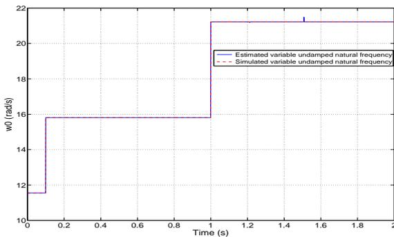
Fig. 16. Algebraic methods estimates for a variable  $\omega_0$
