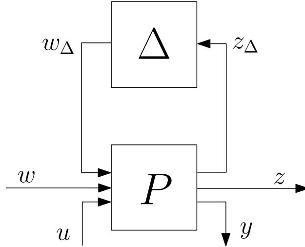
Figure 10: System under LFT form
