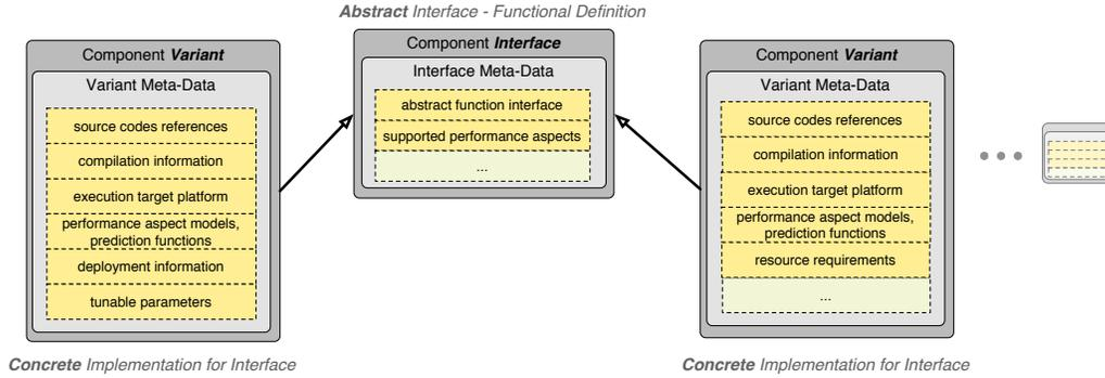
Fig. 2. A PEPPER component consists of an abstract interface describing the functionality of the component, and a number of implementation variants targeted for different architectures and with different performance characteristics. Interface and variant meta-data descriptions are described in XML documents.
