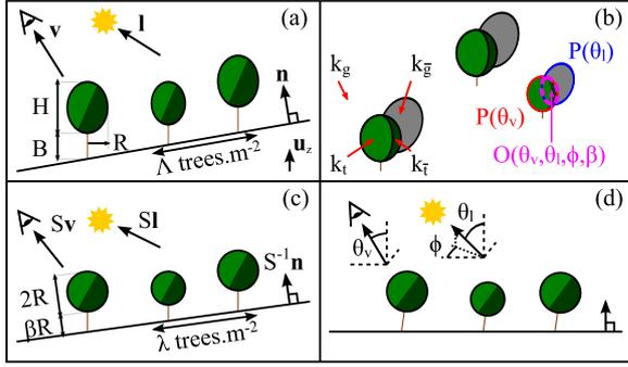
**Figure 2: Strahler et al. model** (from [SJ90, SLS94]). The radiance of a forest patch, modeled with ellipsoids (a), is computed as a weighted sum based on the proportions of sunlit ground  $k_g$ , shadowed ground  $k_{\bar{g}}$ , sunlit crowns  $k_t$  and shadowed crowns  $k_{\bar{t}}$  visible in a pixel (b). A vertical scaling (c) followed by a rotation (d) gives spherical trees on a horizontal ground without changing  $k_g$ ,  $k_{\bar{g}}$ ,  $k_t$  and  $k_{\bar{t}}$ .
