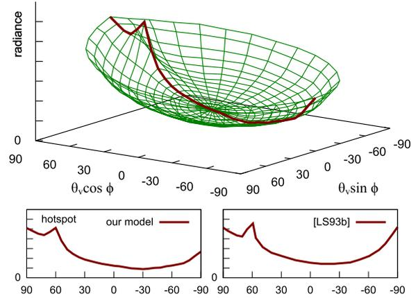
**Figure 8: Validation with reference plots.** The radiance of a forest patch rendered with our method, as a function of the view direction ( $\theta_l = 60$ ). Bottom: with  $r = 0$  as in [LS93b],  $a_1 = 0.2$  and  $a_2 = 20$ , our results are quite similar to theirs.
