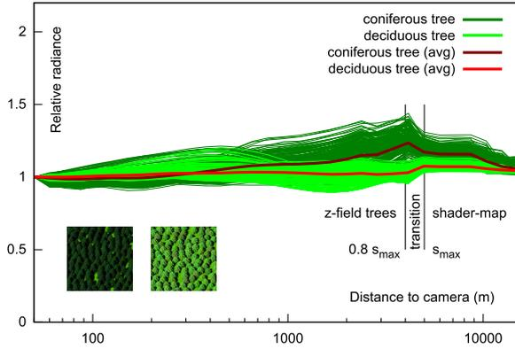
**Figure 7: Validation of scale consistency.** The radiance of a forest patch rendered with our method (insets), as a function of the view distance  $s$ . Each curve shows the ratio  $L(\theta_v, \phi, s)/L(\theta_v, \phi, 50)$  for a different view direction, where  $L(\theta_v, \phi, s)$  is the radiance at distance  $s$  ( $\theta_l = 45$ ). Our results are close to 1, the ideal case where  $L$  is independent of  $s$ .
