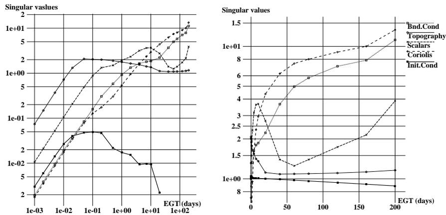
Figure 4: Sensitivity characteristics  $\lambda(t)$  as functions of the Error Growing Time (Log-Log coordinates (left) and Log-Linear coordinates (right)).
