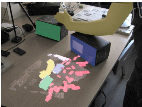
Figure 5: Example of a gaming set. The user puts two boxes (green and blue) to guide incoming creatures (red). He can prevent jumping creatures from getting over the boxes with his arm (yellow).
