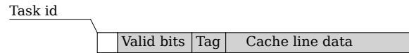
Figure 2: Storage requirements for PRETI caches: each cache line is extended with a task id .
