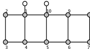
Fig. 4. Coupling topology adapted to 10-8 symmetric characteristics.
