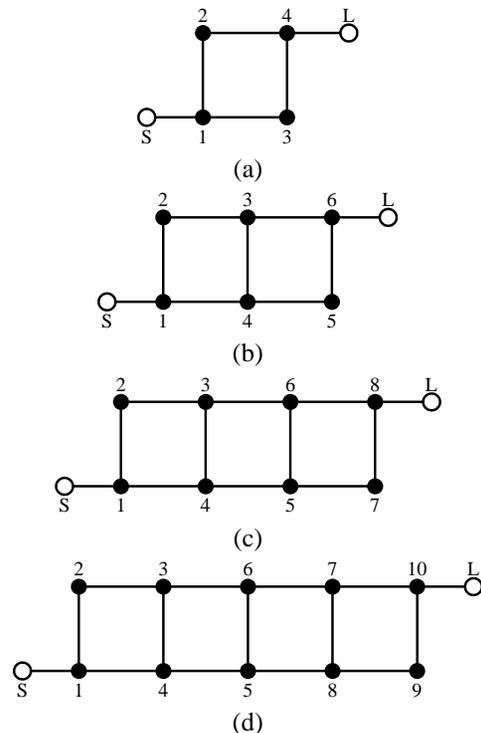
Fig. 1. Coupling and routing diagrams for extended box section networks: (a) 4<sup>th</sup> degree (basic box section) (b) 6<sup>th</sup> degree (c) 8<sup>th</sup> degree (d) 10<sup>th</sup> degree.
