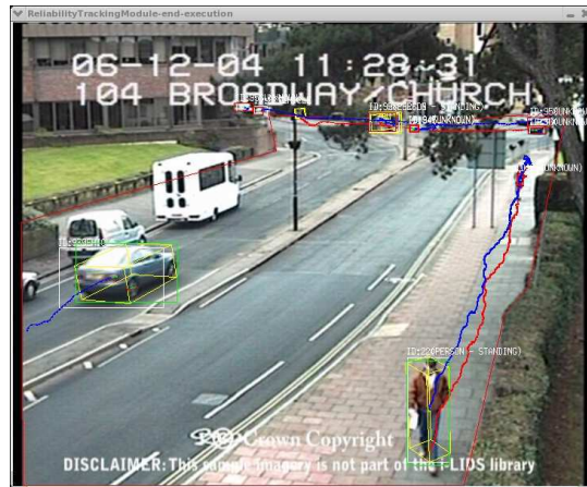
Figure 11 Tracking results for the road video RD-6-C7.
