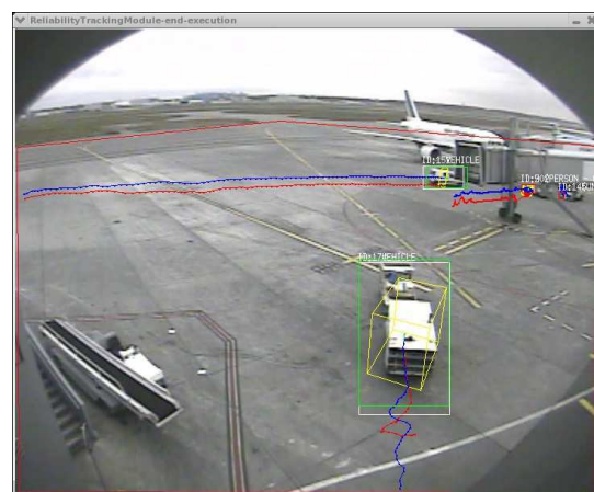
Figure 9 Tracking results for the apron video AP-11-C4.
