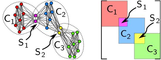
Figure 2: Structure of a decomposable graphical model. **Left:** graph representation. **Right:** corresponding precision matrix. Nodes can be ordered in such a way that they form a succession of cliques  $C_i$ , that are interconnected solely by separating sets  $S_i$ .
