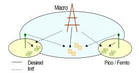
Fig. 1. A heterogeneous network
