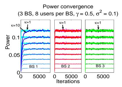
Fig. 2. Power convergence with heterogeneous users
