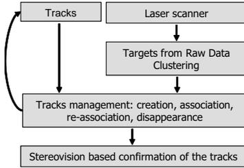
Fig. 2. Overview of the obstacle detection algorithm.
