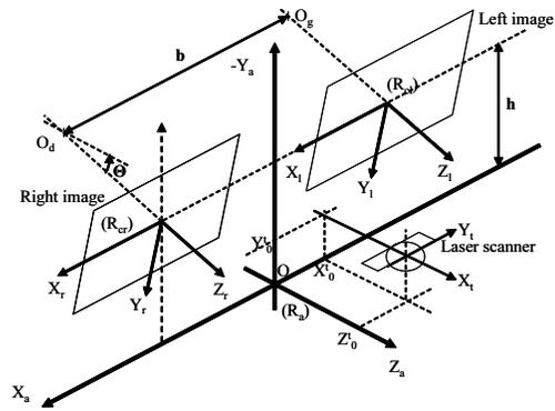
Fig. 1. Geometry of the stereoscopic and laser sensors.
