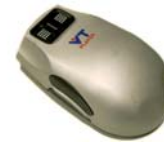
Figure 1. The VTPlayer tactile mouse
