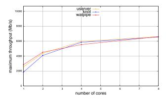
Figure 6. Scalability of the 3 Web servers including NCOPY configura-
