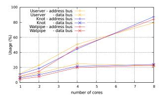
Figure 5. Data and Address bus usage.
