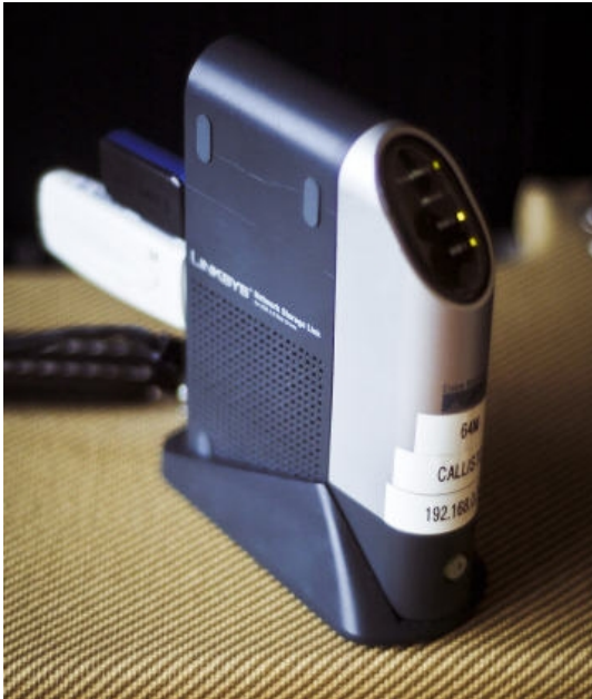
Figure 1: A widrop prototype with Wi-Fi and USB dongles, based on a Linksys NSLU2 flashed with Linux/Debian (2.1 x 9.1 x 13cm dimensions, for a 5 Watts consumption)
