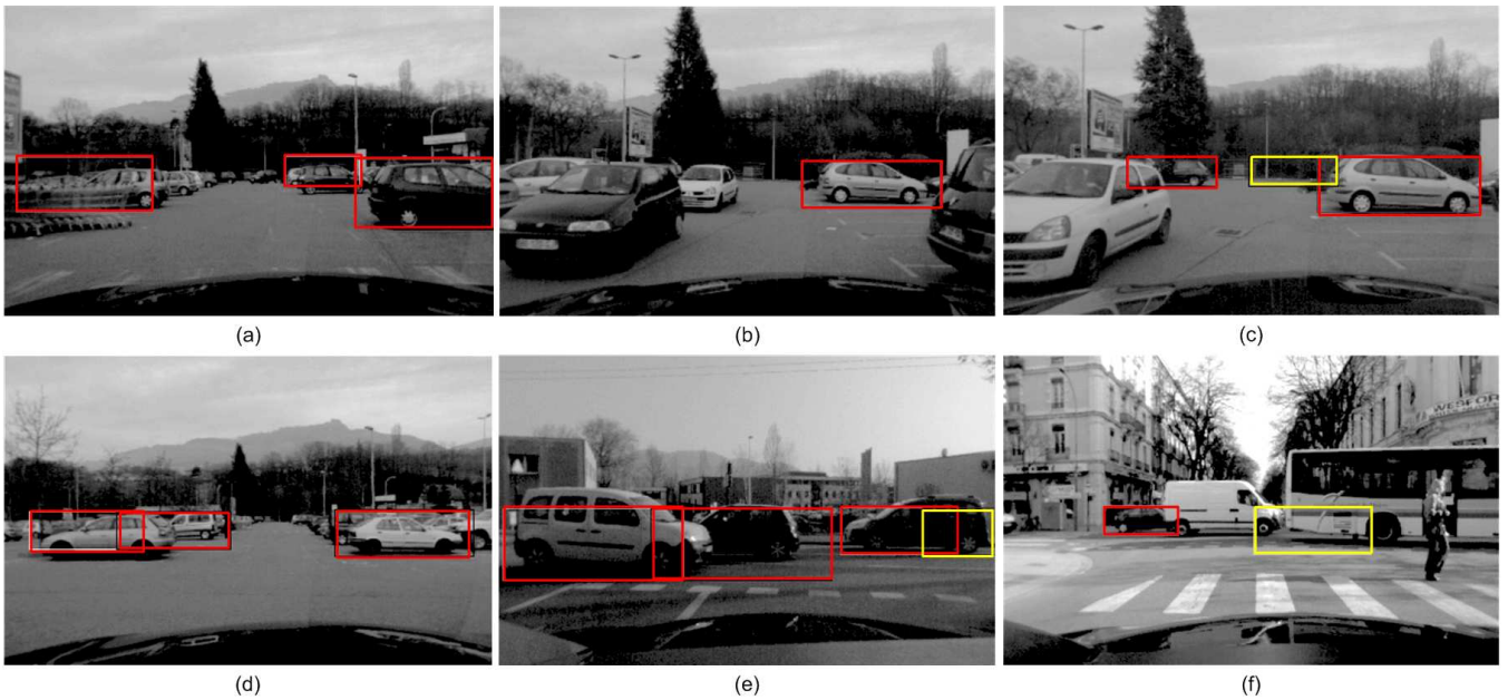
Fig. 6. Car-side detection examples. True and false positive detections are represented with red and yellow bounding boxes respectively. (a) Cars in different scales with significant background clutter and significant occlusions are detected. (b) Precise detection of the un-occluded vehicle, whereas a vehicle that is heavily occluded in the left is not detected. (c) Difficult detection of a vehicle which is far and partially occluded and a false detection in the region between the road surface and the trees. (d) Detection with partial occlusion. (e) Partial detection of a taller than normal vehicle (on the left). The training dataset does not contain vehicles of this type. (f) Successful detection of a partially occluded car and a false positive arising from a bus and a van. Training separate detectors for these type of vehicles as well will help to avoid these false alarms.
