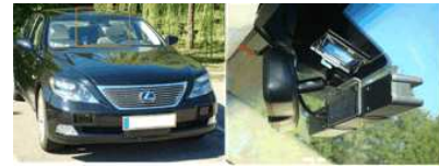
Fig. 5. Our Experimental Platform. Lexus LS600h vehicle equipped with a TYZX stereo camera placed behind the windshield.
