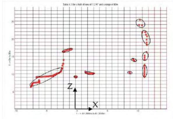
**Fig. 6.** Example of a result of autonomous clustering (a laser point is symbolized by a little circle, and a cluster is symbolized by a black ellipse).
