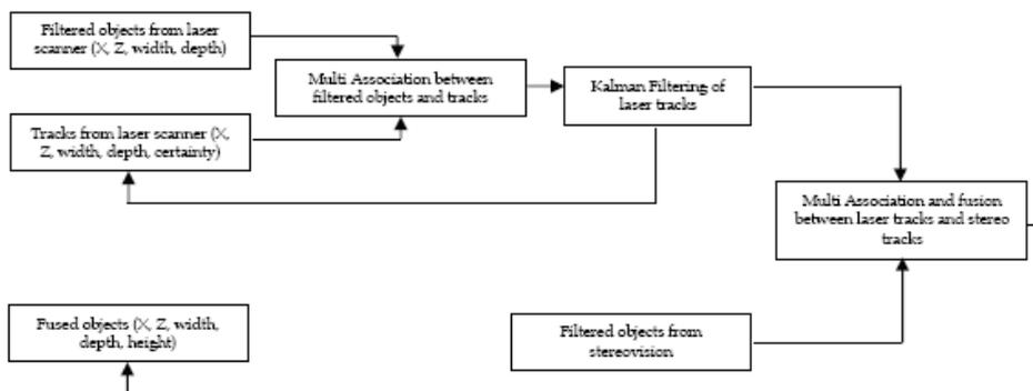
Fig. 12. Fusion with tracking of laser objects.
