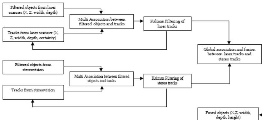
Fig. 11. Fusion with tracking and global association.
