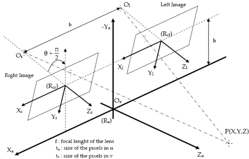
Fig. 1. The stereoscopic sensor and used coordinate systems.
