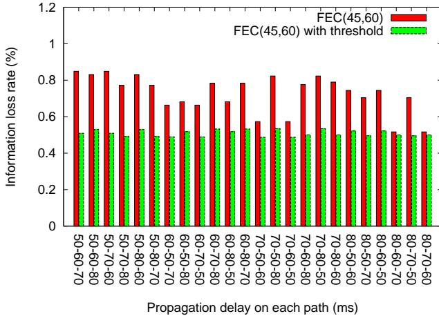
Fig. 8. FEC(45,60) without threshold and with threshold  $\theta = 5\%$  at mean burst size of 2 packets
