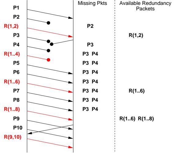
Fig. 2. A simple data exchange with Tetrys ( $k=2$ ) [10]
