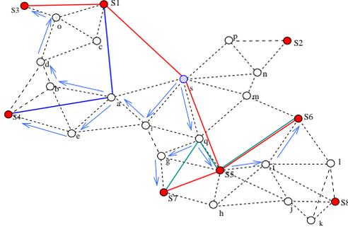
**Fig. 1.** Sinks appear in red. Red links represent the 5-MST rooted in  $s$ , blue links the 2-MST rooted in  $a$  over  $S_1, S_3$  and  $S_4$ , green links the 3-MST rooted in  $q$  over  $S_2, S_5, S_6, S_7$  and  $S_8$ . Arrows show the message path.
