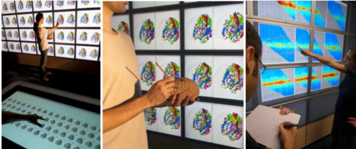
Figure 3: Interaction instruments. (left) An interaction instrument sorts the 64 displayed brain scans, (center) a brain prop controls the scan orientation, and (right) a digital pen annotates content on the wall. (Source: Photothèque CNRS, Cyril Fresillon.).
