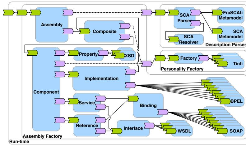
Figure 6: Architecture of the FRASCATI Assembly Factory.
