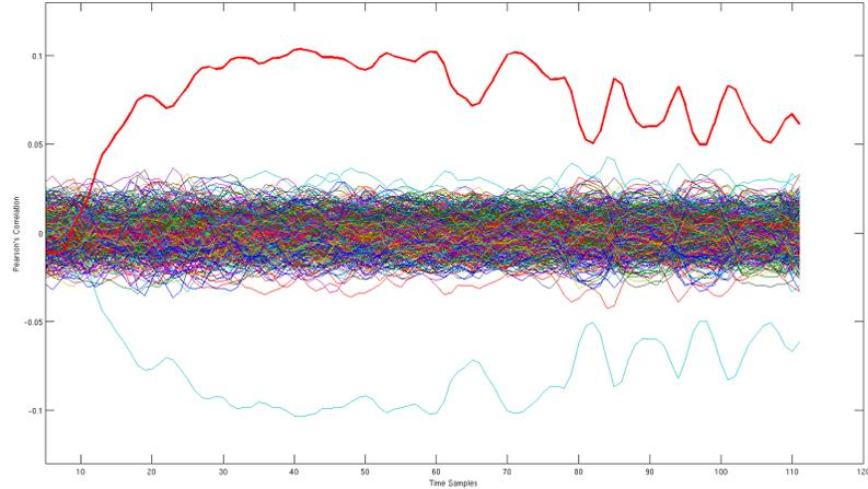
**Fig. 4.** SCARE on the 7<sup>th</sup> component of  $\mathcal{SB}^{-1}$ , with  $N = 10000$  power traces. We have the 510 correlation traces: on the x-axis the time samples of the power traces, on the y-axis, the value of the correlation. We clearly identify here the solution (on the top) and its complementary (on the bottom)
