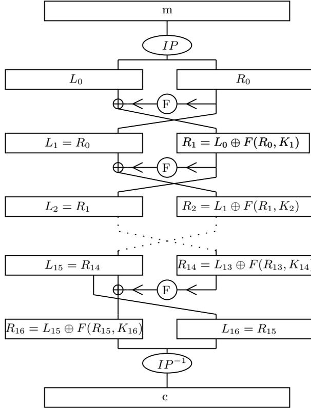
**Fig. 1.** The DES cipher, a 16-round Feistel cipher.  $IP$  is a 64 bit permutation. The round function applies  $F$  to the right half of the register, XORs the result to the left half, and exchanges the roles of the halves.
