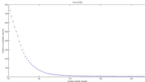
**Fig. 2.** Attacking component 0 of the first S-Box of DES: On the x axis, the number of faults injected, on the y-axis the mean of  $\#\mathcal{L}_{1,0,x}$  after 1000 tries. In the end, we only have 2 candidates.
