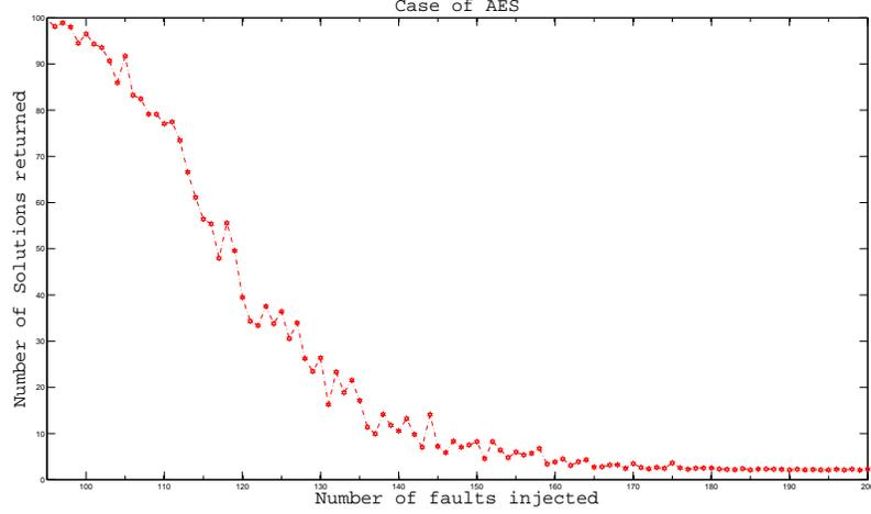
**Fig. 5.** Attacking component 0 of AES S-Box inverse. On the x-axis, the number of faults injected, on the y-axis the mean of  $\#\mathcal{L}_{0,x}$  after 100 tries. In the end, we only have 2 candidates.
