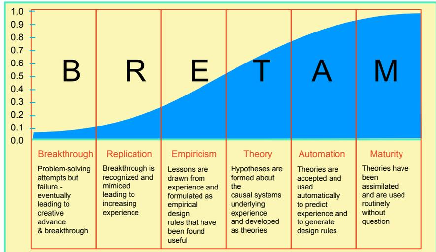
Figure 6.1: The BRETAM sequence plotted along the underlying logistic learning curve<sup>[6]</sup>
