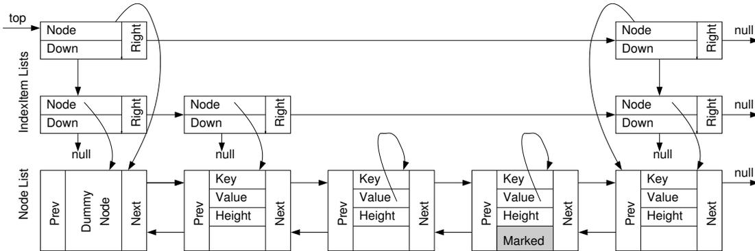
Figure 2: The contention-friendly non blocking skip list structure
