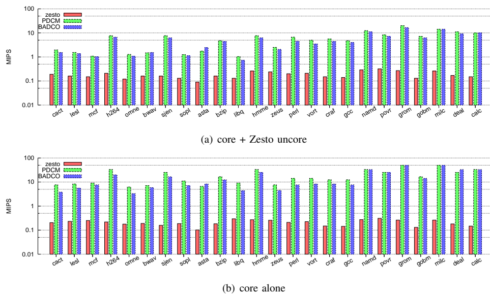
Figure 6. Simulation speed in millions of instructions simulated per second (MIPS) with and without considering the impact of the Zesto uncore (logarithmic scale).
