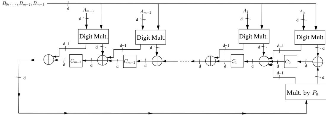
The complexity of this digit sequential multiplier is given below. Note that  $\mathcal{S}_{\oplus}$  represents the number of XOR gates,  $\mathcal{S}_{\otimes}$  represents the number of AND gates and  $\mathcal{D}$  represents the delay of the critical path of the architecture. We remark that the total computational delay is the number of clock cycles times the clock period, whose duration is at least the critical path delay.
