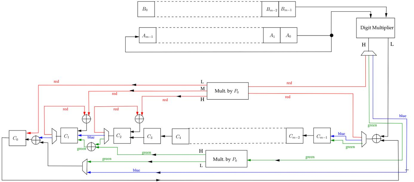
and XOR gates and the critical path of the architecture in terms of  $m$  and  $d$ . For the sake of simplicity, we assume that each path in Fig. 2 is of width  $d$ .
