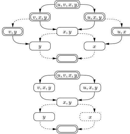
Figure 4: Micro-step automata encoding causality equations  $x \leftarrow u \wedge y \leftarrow v$  (top) and  $(x, y) \leftarrow (u, v)$  (bottom). For both STS,  $u, v$  are declared inputs and  $x, y$  are declared outputs. With the partitioning of transitions as solid/dashed and of states as marked/unmarked, we get Convex Acceptance Interfaces introduced below.
