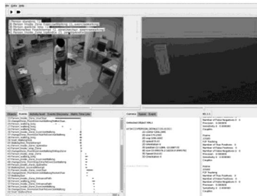
Figure 1. Multi-sensors monitoring system results being analyzed in the evaluation platform (VISEVAL)
