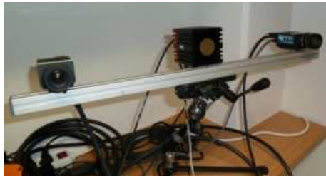
(a) A TOF-stereo setup
