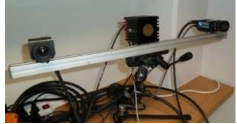
(a) A TOF-stereo setup
