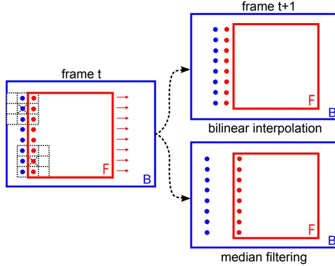
Figure 4: Comparison of bilinear interpolation and median filtering. The object is moving to the right. Pixels along the motion boundary are indicated by the blue and red dots. The blue dots belonging to the background should stay in place, whereas the red dots should follow the moving foreground object. Using bilinear interpolation, motion boundaries are blurred, and thus foreground and background motion information are confused. Median filtering allows to maintain a sharp motion boundary.
