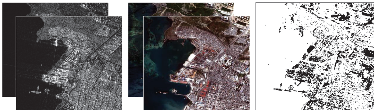
Fig. 1. CD results with multitemporal CSK® (left; COSMO-SkyMed Product – ©ASI – Agenzia Spaziale Italiana – 2009-2010) and QuickBird images (center; ©DigitalGlobe, 2011) acquired over Port-au-Prince (Haiti) before and after the 2010 earthquake. Black and white in the change map (right) denote “change” and “no-change,” respectively.
