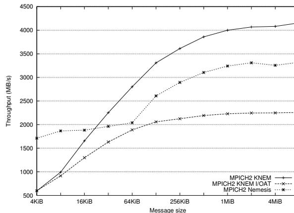
Figure 12: Comparison between IMB Pingpong throughputs using the native MPICH2/NEMESIS implementation, MPICH2 over the KNEM LMT, and MPICH2 over KNEM with I/O AT copy offload, on a dual-socket INTEL *Westmere* platform (Figure 8(a)), with no cache reuse and different sockets.
