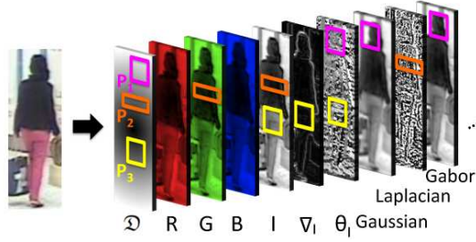
Fig. 1. A meta covariance feature space. Example of three different covariance features. Every covariance is extracted from a region ( P ), distance layer ( \mathfrak{D} ) and three channel functions ( e.g. bottom covariance feature is extracted from region P_3 using layers: \mathfrak{D} , I -intensity, \nabla_I -gradient magnitude and \theta_I -gradient orientation).
